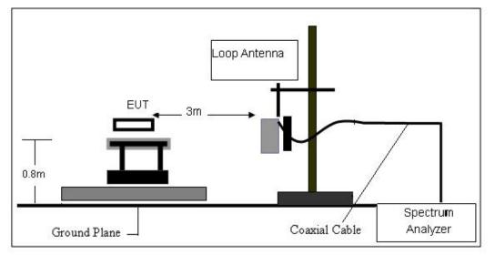
(B) Radiated Emission Test-Up Frequency 30MHz~1GHz
