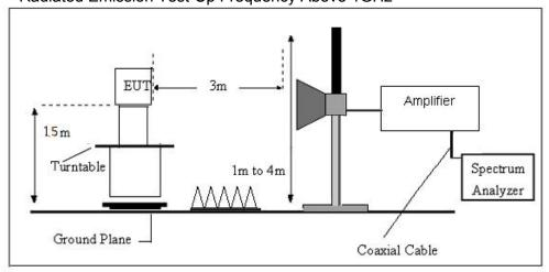
Radiated Emission Test-Up Frequency Above 1GHz
