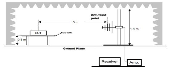
(B) Radiated Emission Test-Up Frequency 30MHz~1GHz
