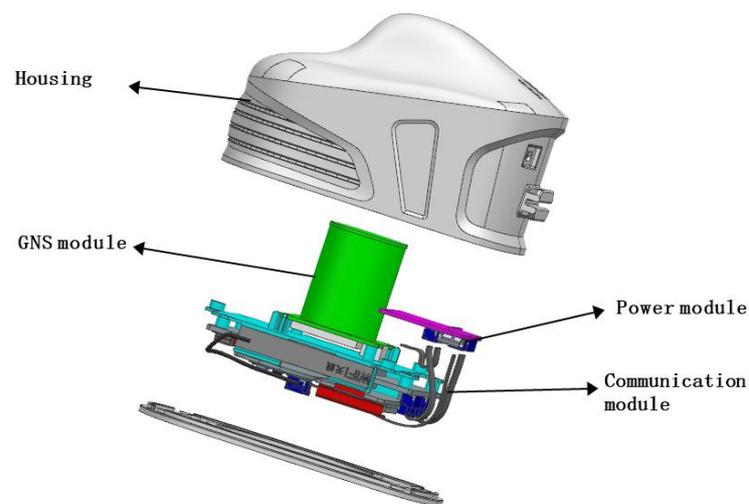
1. **Housing:** Use the plastic material to make sure the signal quality of the GNSS system.
