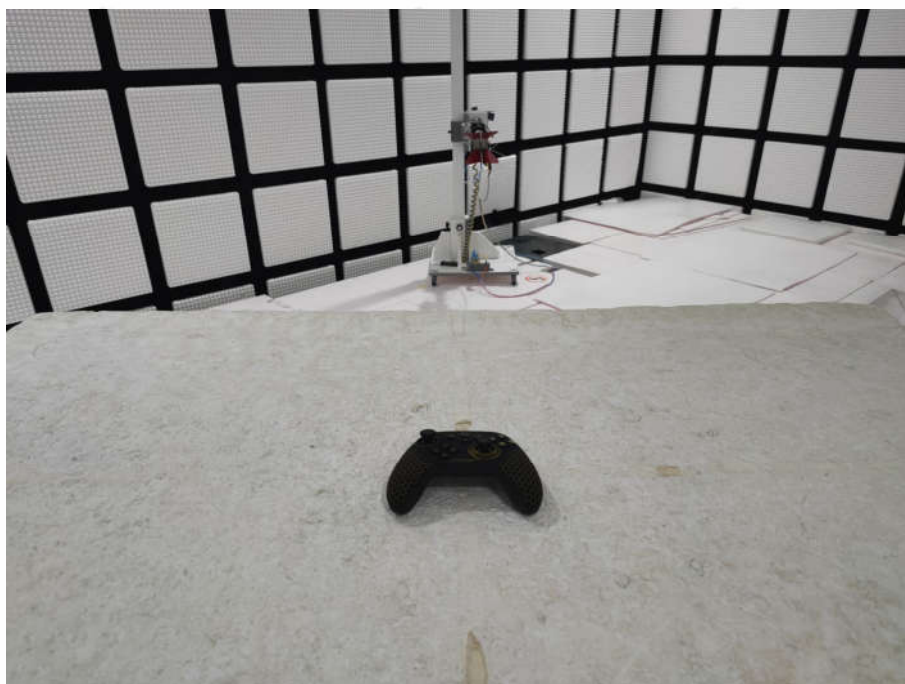
Radiated spurious emission Test Setup-2(Above 1GHz)
