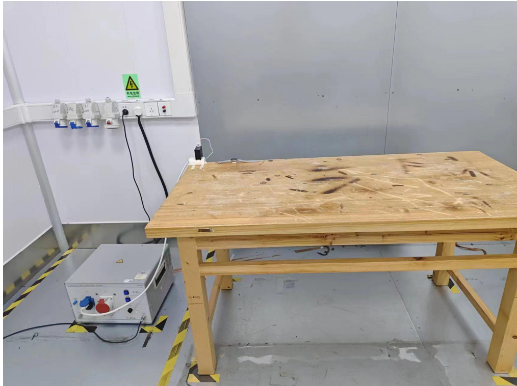
Conducted Emission at AC power line
