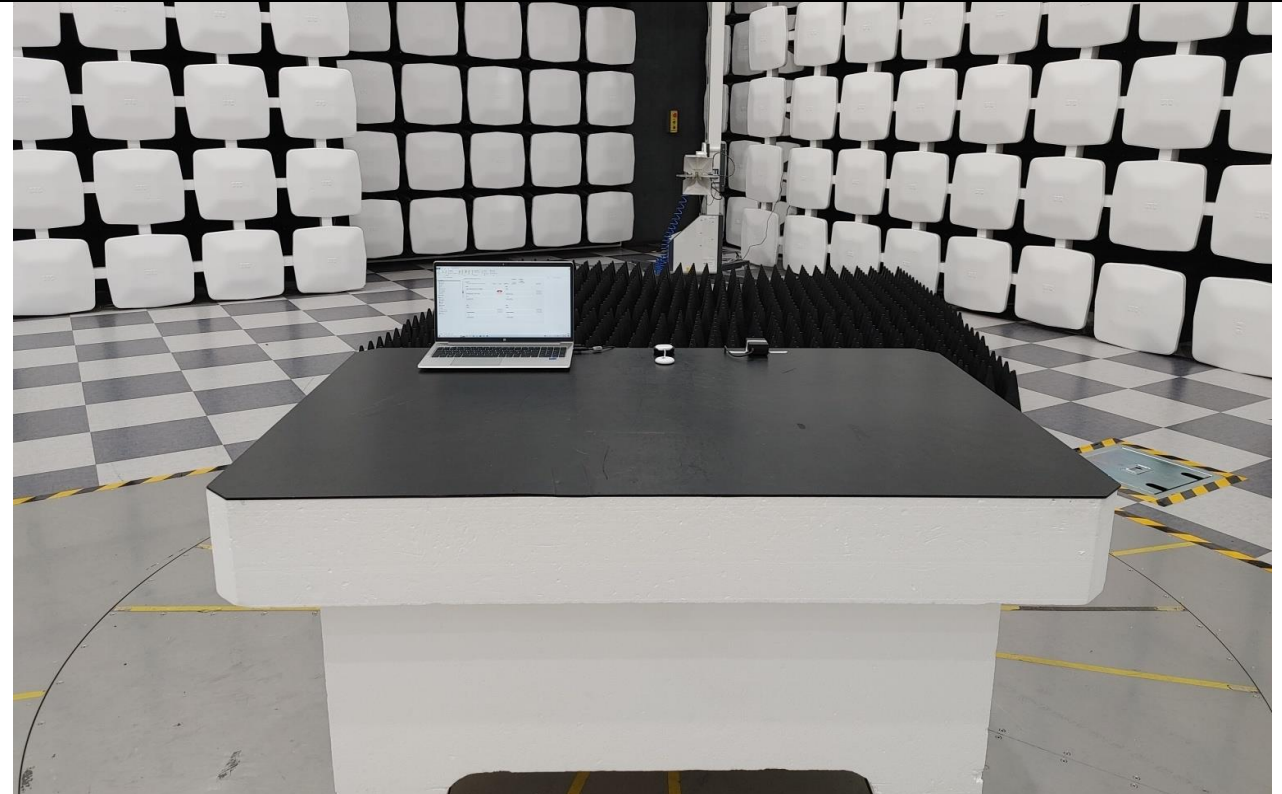
Photo of test set up for radiated emissions Test configuration: Configuration 1 (Data transmitting) [Above 1 GHz]
