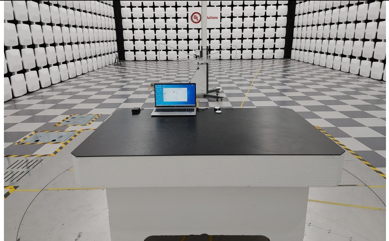
Photo of test set up for radiated emissions Test configuration: Configuration 1 (Data transmitting) [Below 1 GHz]
