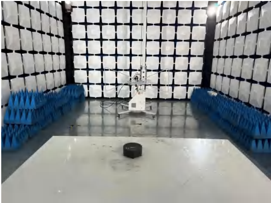
Above 1GHz for radiated emission test setup
