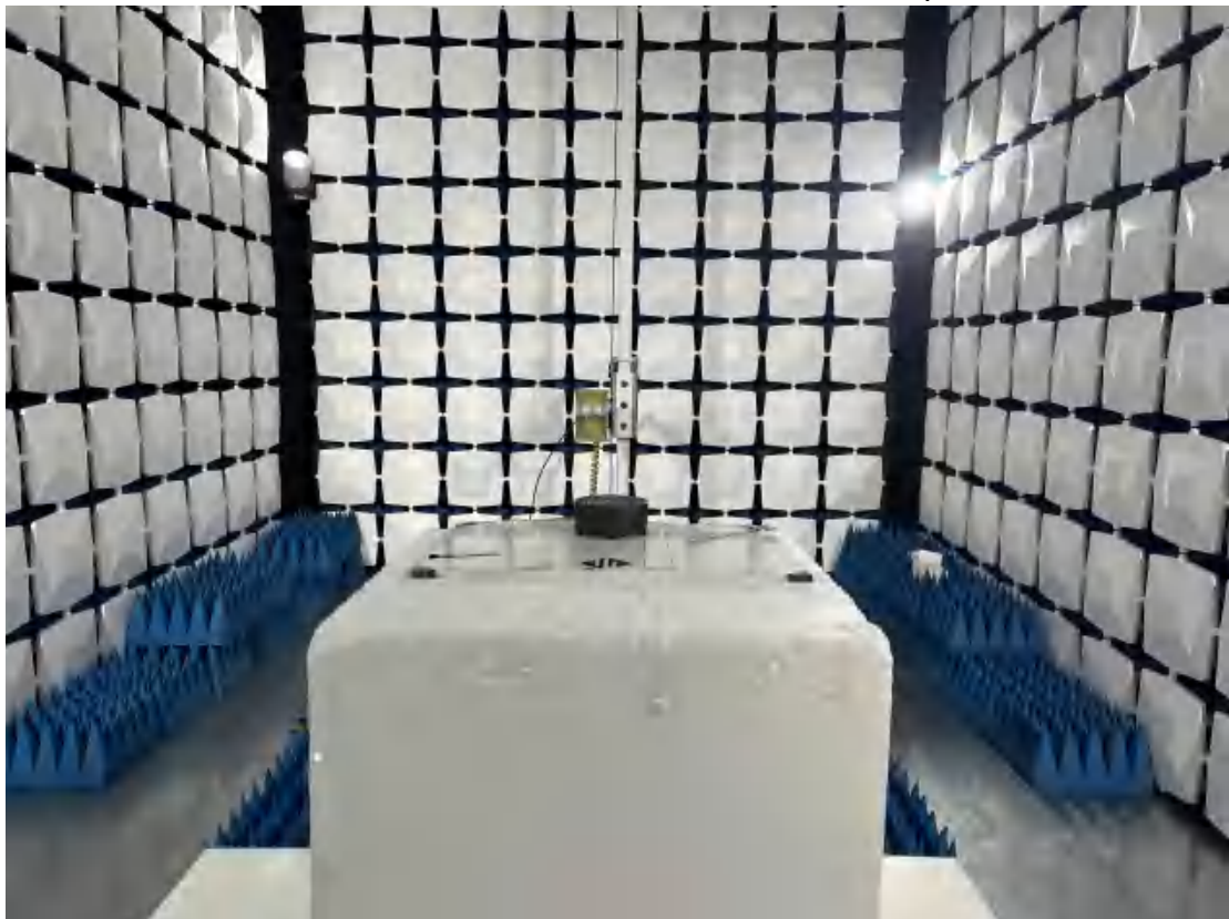
Above 1GHz for radiated emission test setup
