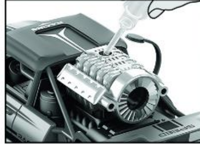
OPEN THE WATER INJECTION PORT AND INJECT CLEAN WATER
