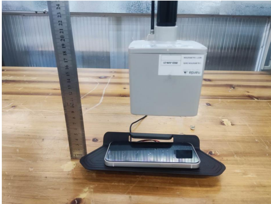
Test Position E-15cm from the edge of EUT to the geometric center of the probe
