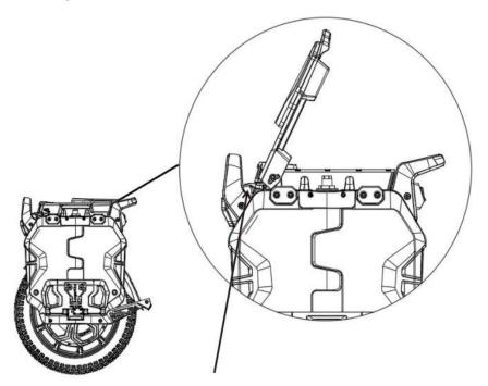
Move pick upward to switch seat and trolley handle.
