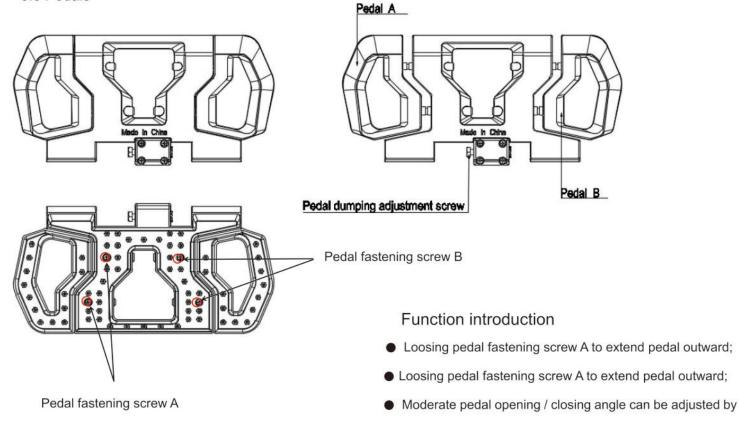
right turning the pedal damping screw.
