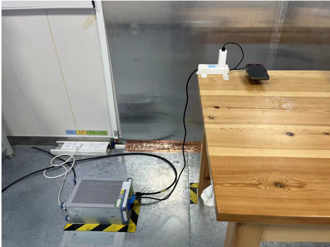
Conducted emission test setup
