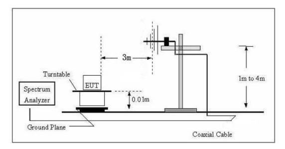
(C) For radiated emissions above 1000MHz
