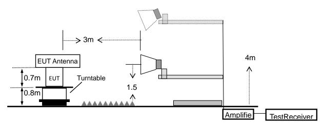
Note: the antenna of the EUT was located at a height of 1.5 m above the floor.
