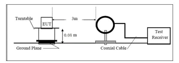
(B) For radiated emissionsfrom 30MHz to 1000MHz
