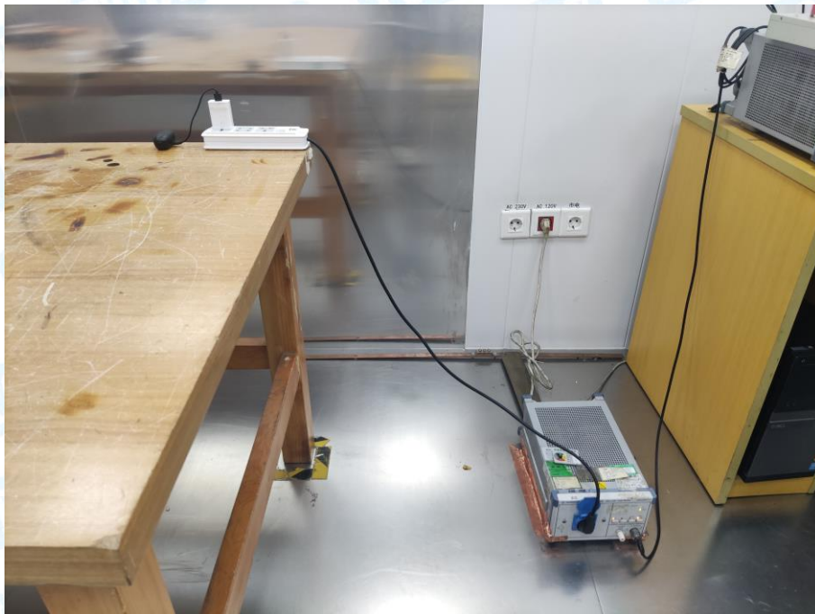
Photo of Setup for Conducted Emission
