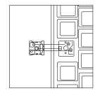
3.Align the new keyswitch's pins and base
