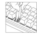
2.Position the tips of the keyswitch puller under the keyswitch top and bottom tabs, then press in and lift to remove
