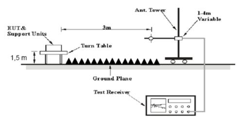
The radiated emissions were performed in the 3 meters distance, using the setup accordance with the ANSI C63.10-2013. The specification used was the FCC 15.209, and FCC 15.249 limits.
