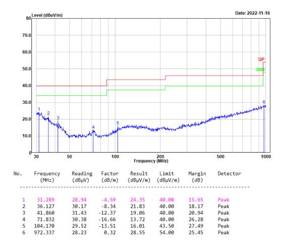
Test Mode: Transmitting Polarization: vertical
