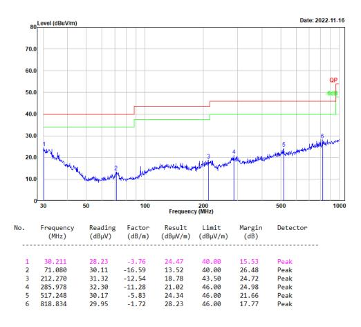
Test Mode: Transmitting Polarization: vertical Note:
