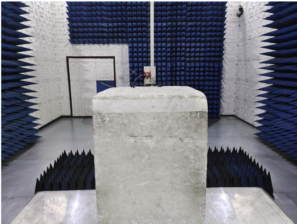
RADIATED EMISSION TEST SETUP ABOVE 1GHz
