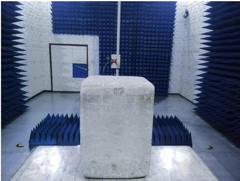
RADIATED EMISSION TEST SETUP ABOVE 1GHz
