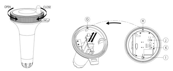
After disassembly, do not touch other components, especially the antenna "I", pay attention to the direction of the slot when installing the battery box. After setting, align "H" with "G", cover the lens and waterproof ring, and lock the cover tightly.
