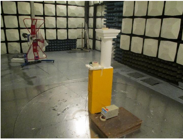
Test Setup – Radiated emission from 1 GHz to 18 GHz
