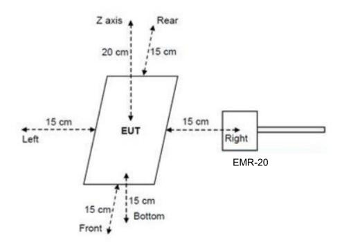
4.4. Block Diagram of Test Setup
