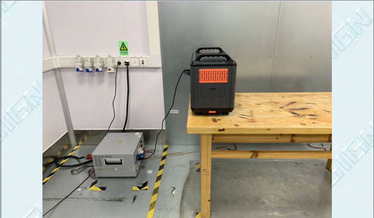
Conducted Emission at AC power line
