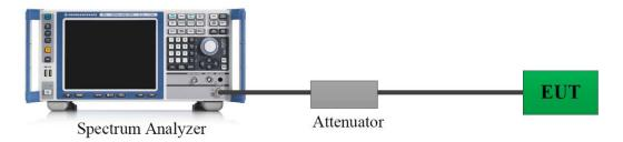
A short RF cable with low cable loss connected to the EUT antenna port, which was provided by manufacturer.
