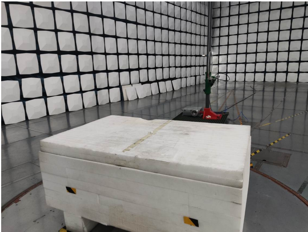
Radiated Emission 9k-30MHz Perpendicular View
