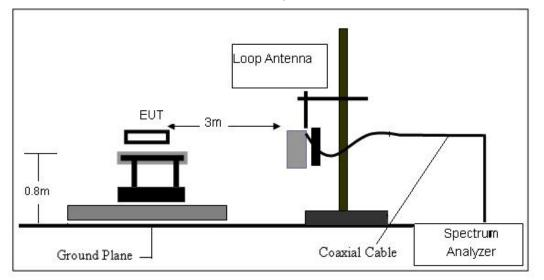
(B) Radiated Emission Test-Up Frequency 30MHz~1GHz
