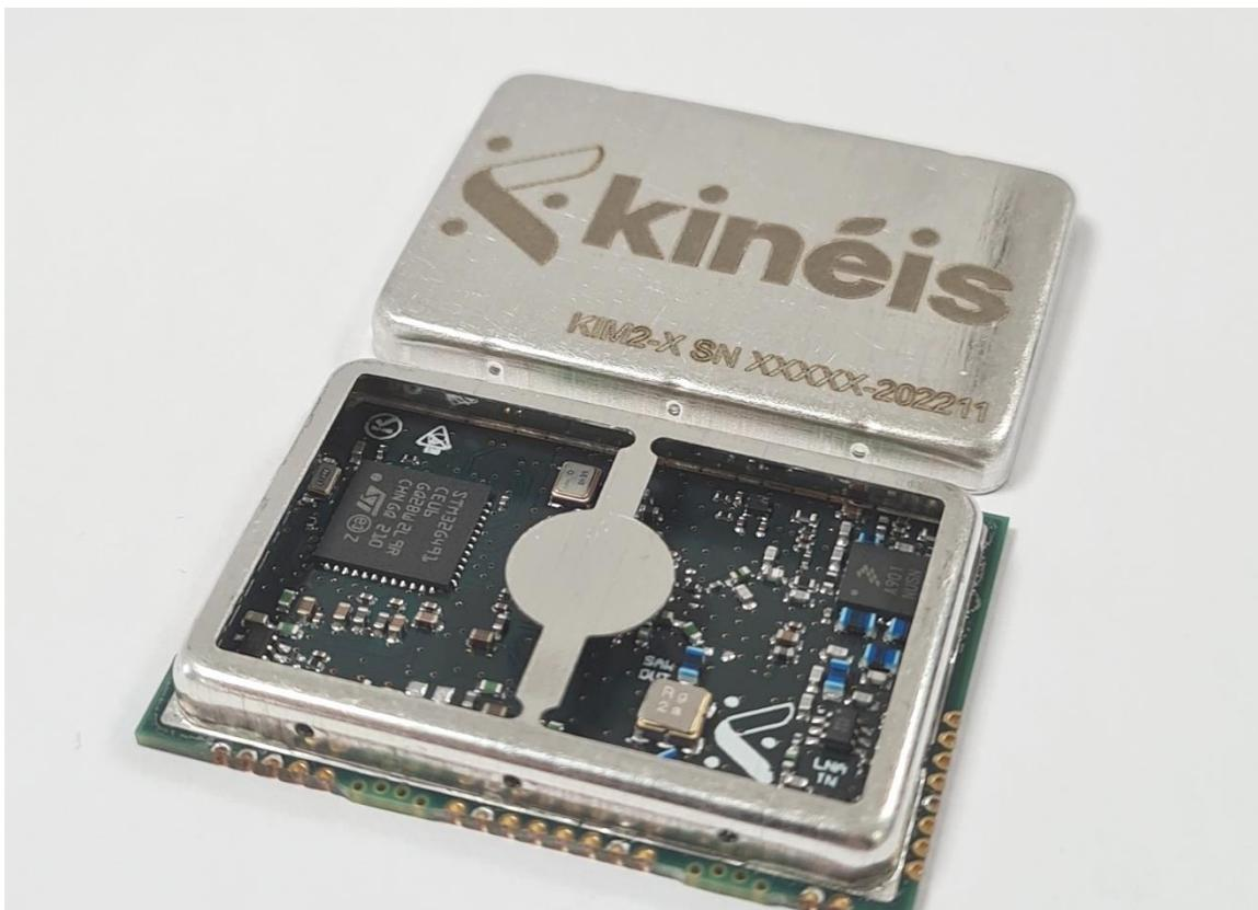
Here is a top view of the module without neither the frame nor the shield:
