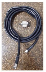
As, the interface board connector and antenna connectors are not compatible, it is required to use a SMA/N-type adapter.
