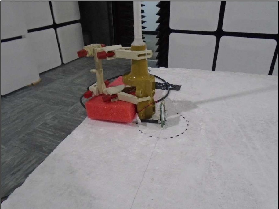
Figure 10 - Dipole Stick Antenna, Orientation Z
