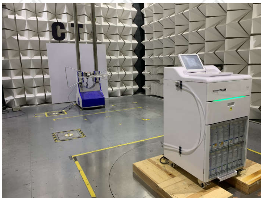
Radiated Spurious Emissions Test Setup (30MHz~1GHz)
