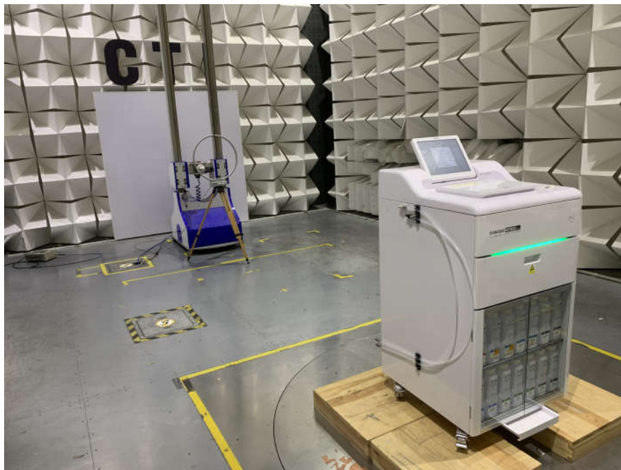
Radiated Spurious Emissions Test Setup (9kHz~30MHz)
