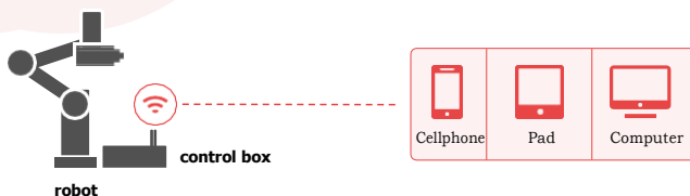
Figure 2.3 Wireless network connection topology diagram
