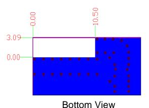
Transmission Line with 50Ω Impedance Characteristic
