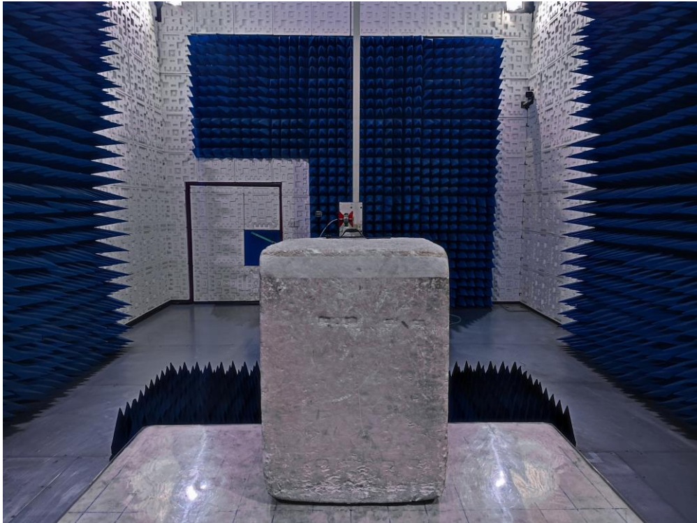
RADIATED EMISSION TEST SETUP ABOVE 1GHz
