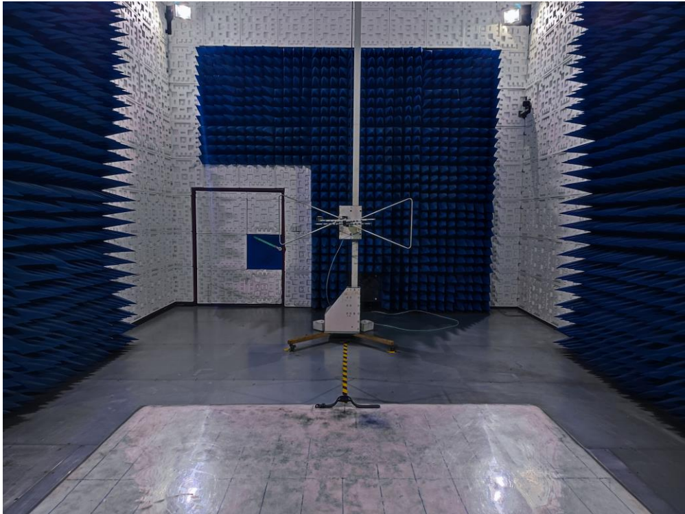
RADIATED EMISSION TEST SETUP ABOVE 1GHz
