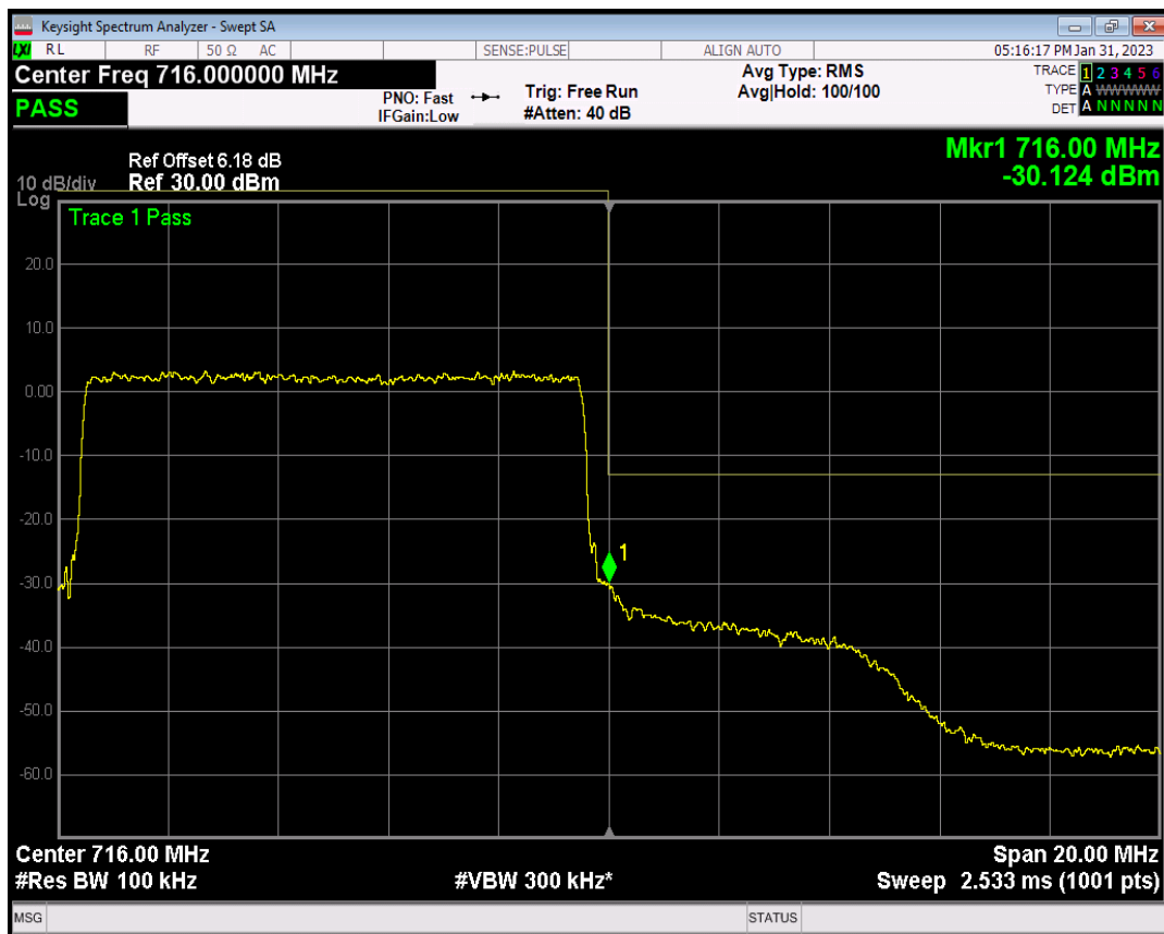
Band2 QPSK BW=1.4MHz Channel=18607 RB Size=1 Position=#0
