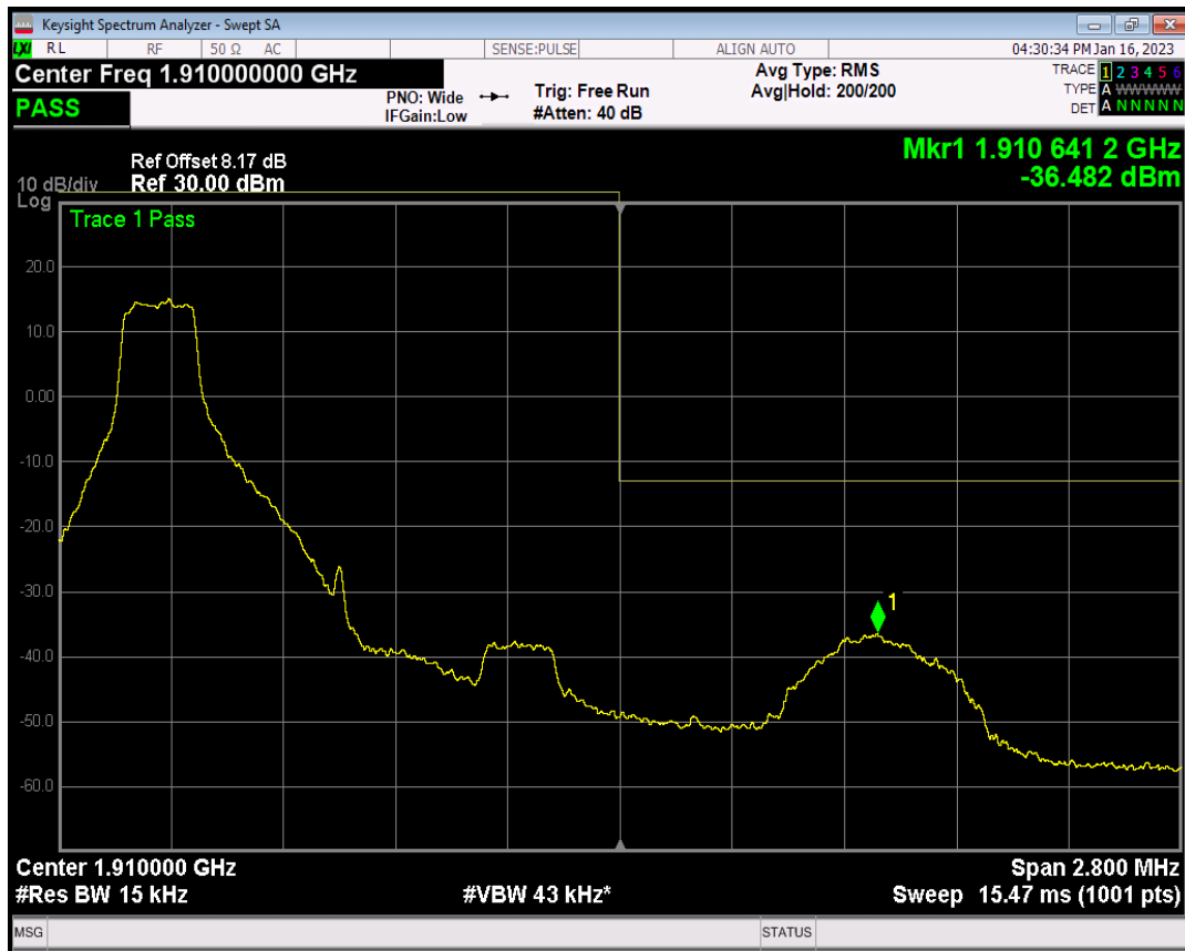
Band2 QPSK BW=1.4MHz Channel=19193 RB Size=1 Position=#Max
