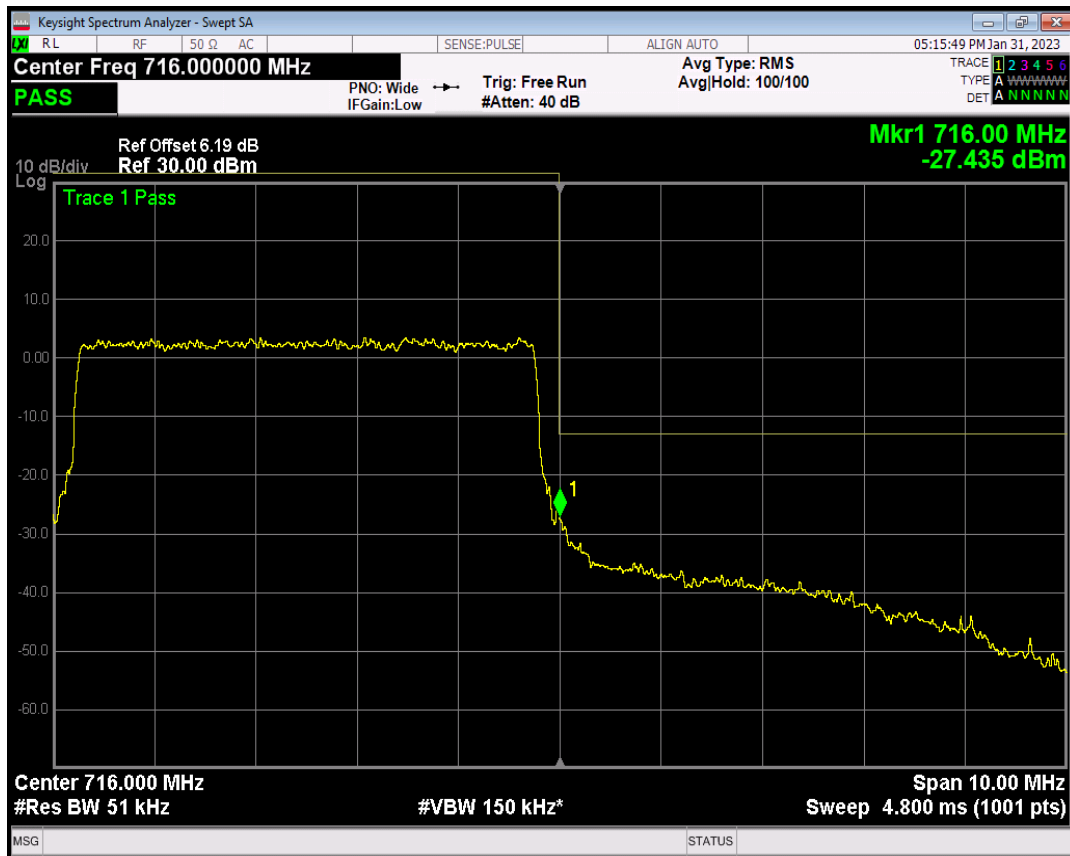
Band17 QPSK BW=10MHz Channel=23780 RB Size=1 Position=#0
