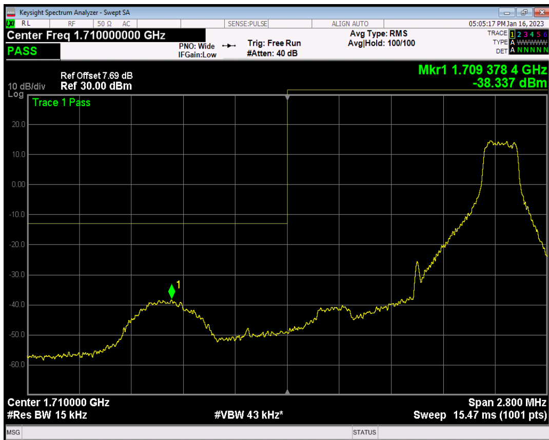
Band4 QPSK BW=1.4MHz Channel=19957 RB Size=6 Position=#0
