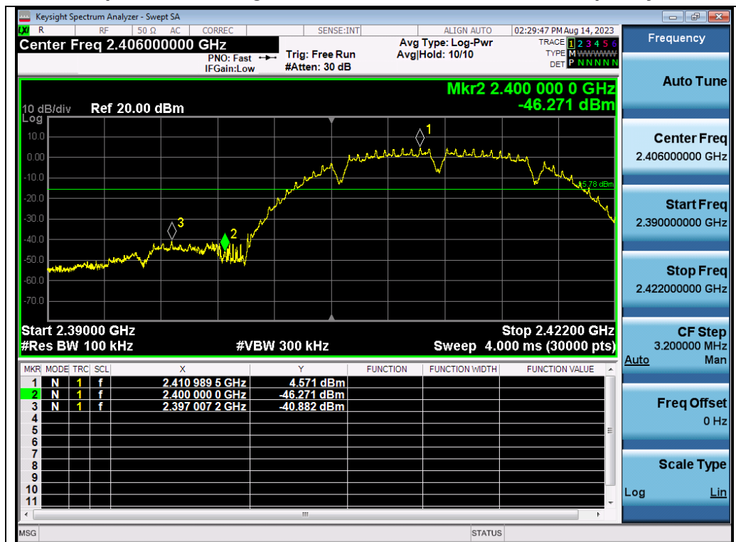
Test_Graph_802.11b_ANT1_2412_1Mbps_Lower Band Edge Emissions
