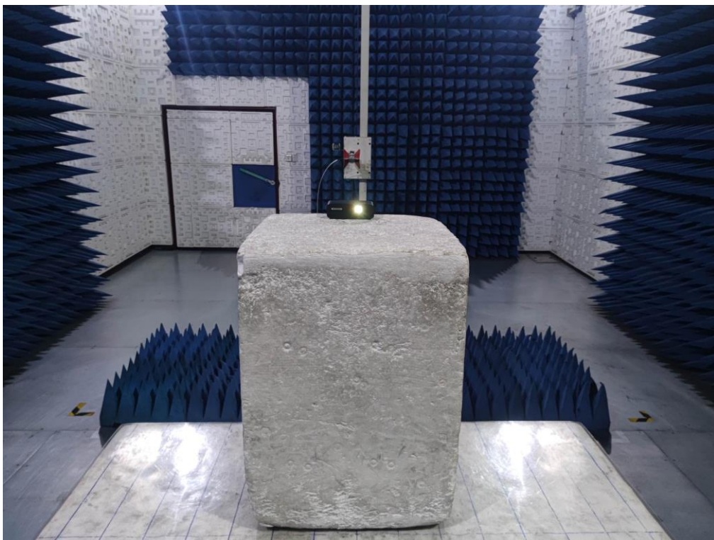
RADIATED EMISSION TEST SETUP ABOVE 1GHz
