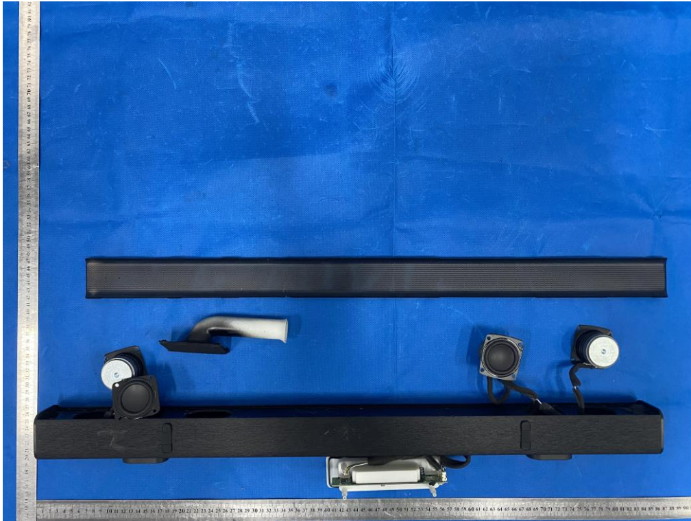
INTERNAL VIEW OF EUT (FIGURE 1)
