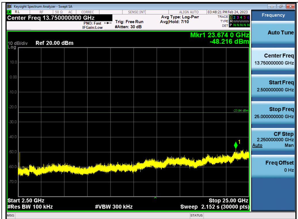
Test_Graph_BR_ANT1_2480_1Mbps_Higher Band Emissions
