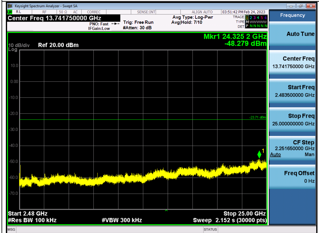
Test_Graph_EDR_ANT1_2402_2Mbps_Higher Band Emissions
