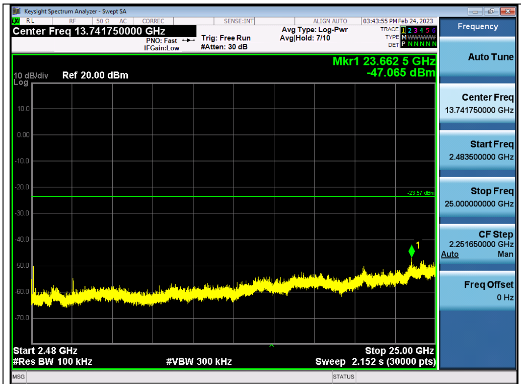
Test_Graph_BR_ANT1_2402_1Mbps_Higher Band Emissions
