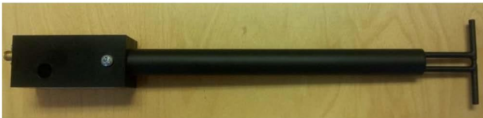
Figure 1 – MVG COMOSAR Validation Dipole
