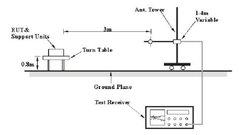
The radiated emission tests were performed in the 3-meter chamber test site, using the setup accordance with the ANSI C63.10-2013. The specification used was the FCC Part Subpart C limits.
