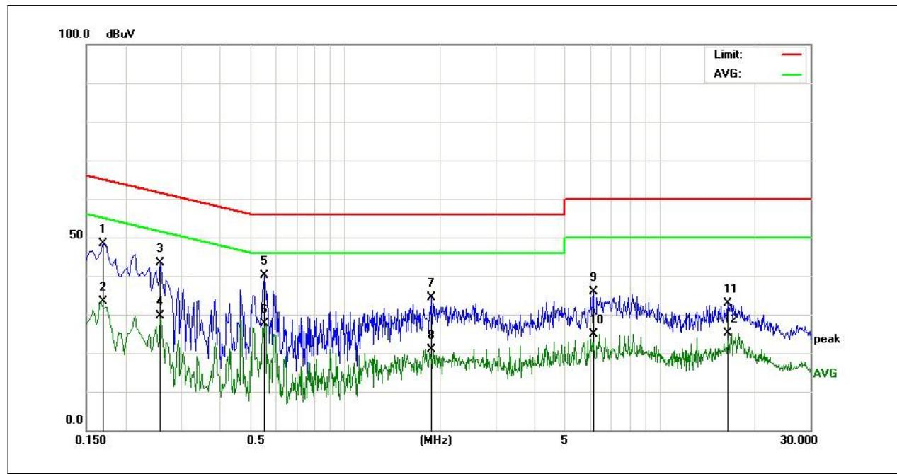
Remark: Factor =insertion loss of LISN + Cable loss +insertion loss of Pulse Limiter +insertion loss of Switch.
