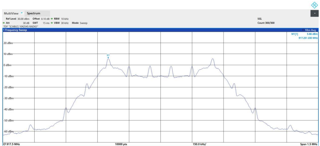
Fig. 18: Low Channel - Power Spectral Density
