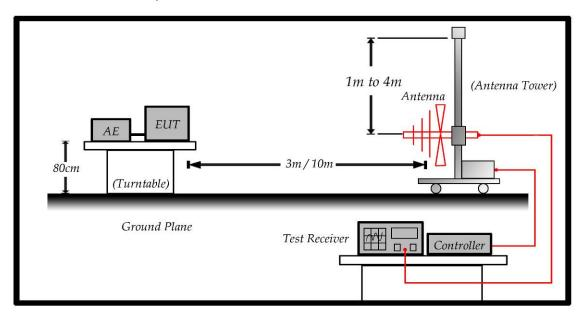
Above 1GHz Test Setup:
