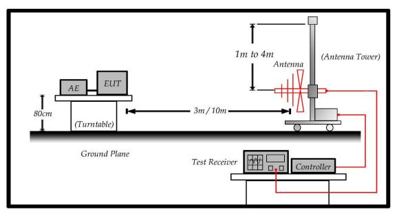
Above 1GHz Test Setup:
