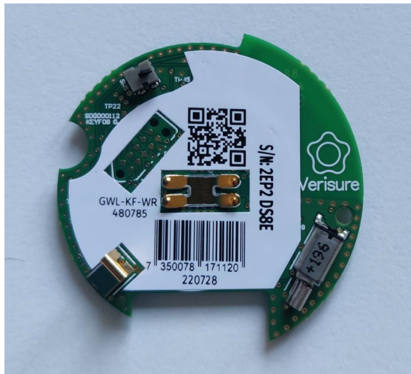
Figure 5 KeyFob PCB bottom
