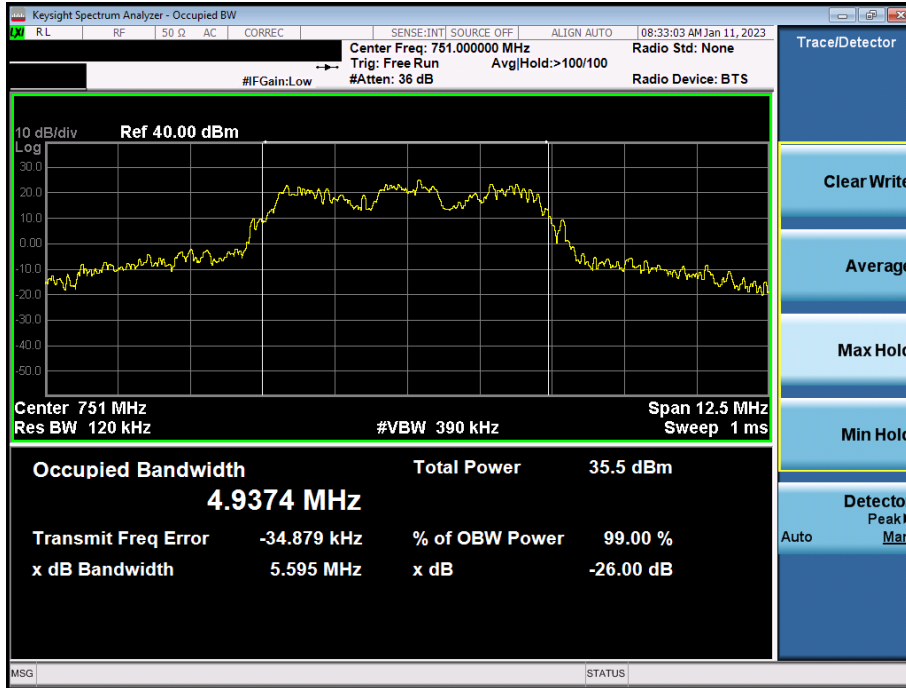
Plot 7-12. Occupied Bandwidth Plot (LTE Band 13 - 5MHz- Full RB)
