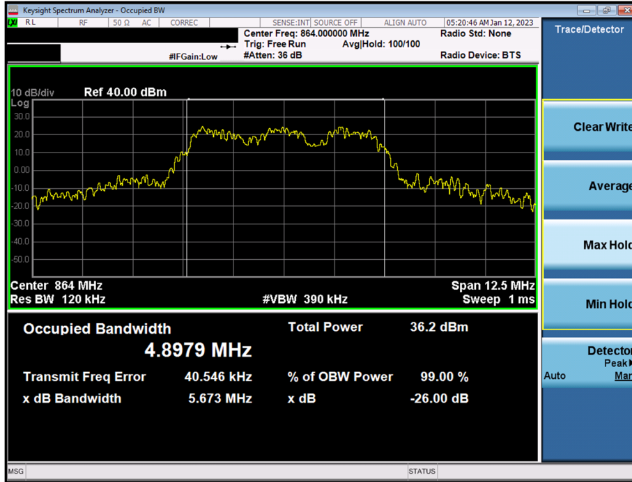
Plot 7-3. Occupied Bandwidth Plot (LTE Band 26 - 5MHz - Full RB)
