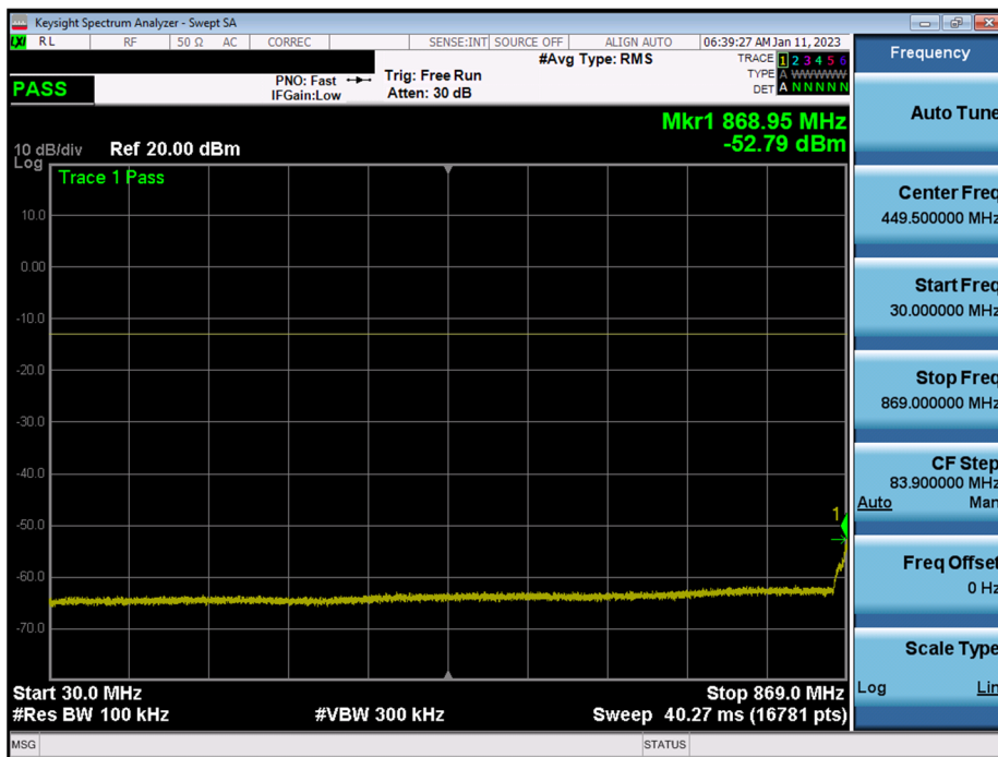
Plot 7-8. Conducted Spurious Plot (LTE Band 26 - 5MHz QPSK – Full RB - Mid Channel)
