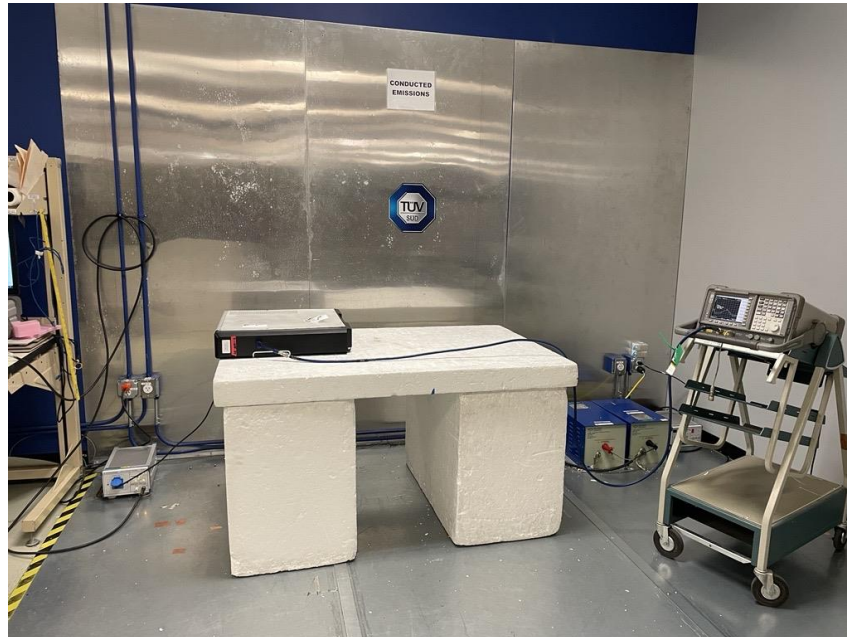
Figure 3 – Test Set up – Power Line Conducted Emissions
