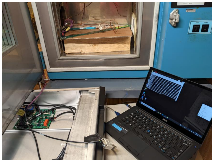
Figure 4 – Test Set up – Frequency Stability Measurement
