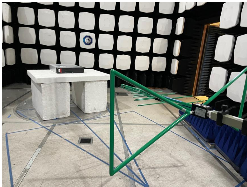
Figure 2 – Test Set up - Radiated Emissions <1 GHz
