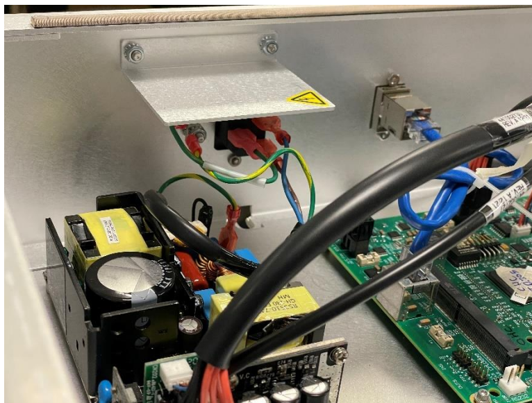
Figure 1.6-2 – Removed Schaffner FN9222-15-06 inlet filter
